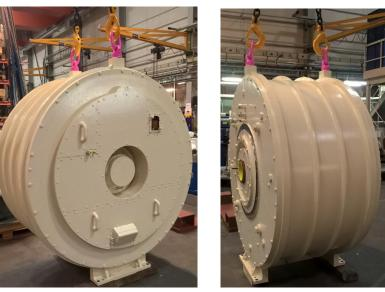
XT140 is an electrical motor with a large diameter and large output torque. The motor is designed as a permanent magnet motor controlled by a frequency drive.
